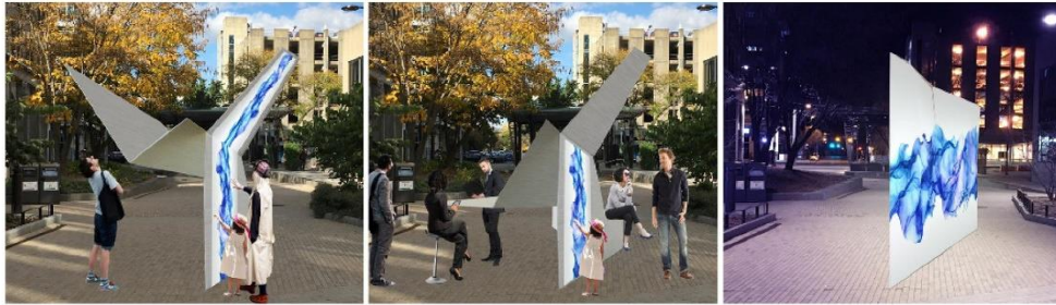
Fig. 9: A case study of the vertex pop-up mechanism, transFORM (three configurations shown above) is 2.5m (approx. 8ft) tall in its flattened configuration (the right-most image, shown at night).
