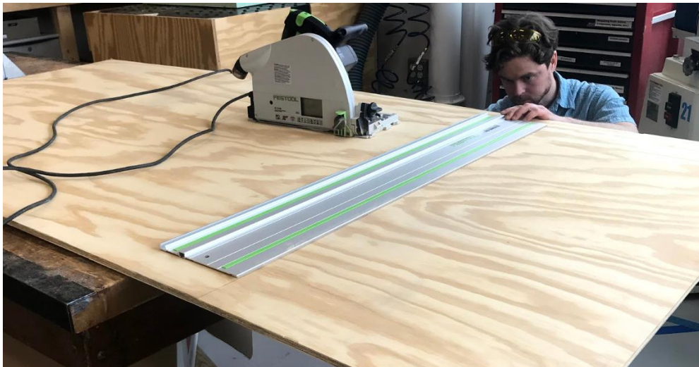
Figure 25 – Foot fabrication from construction-grade plywood.
