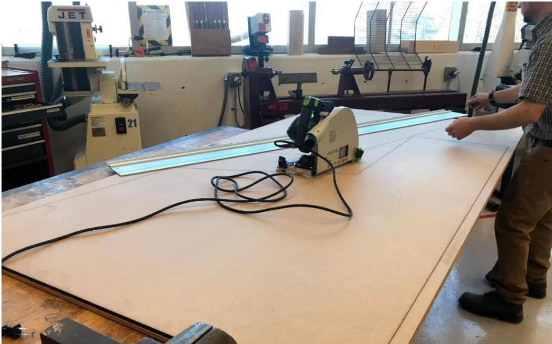
Figure 23 – Cutting the MDF panels using a circular saw.
